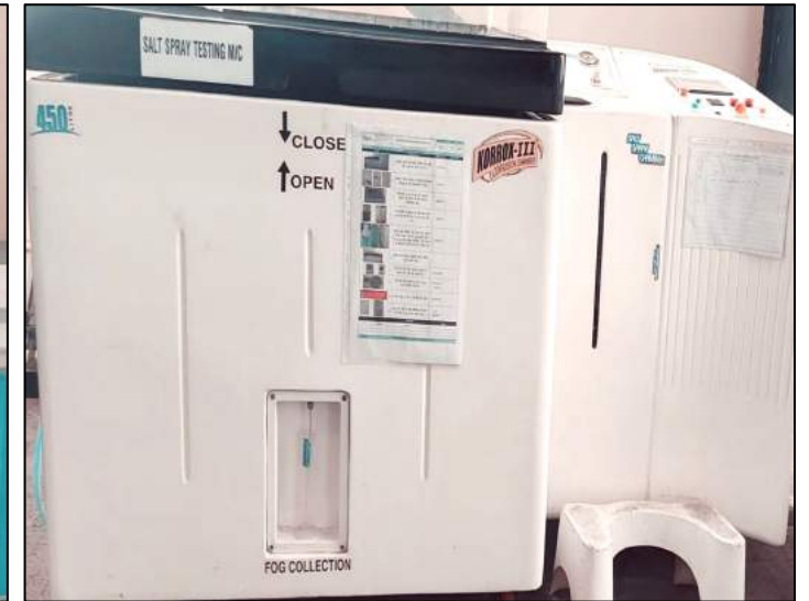
Salt Spray Test
