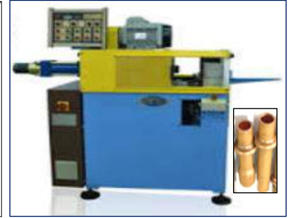
Pipe End Forming With Spinning
